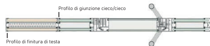
Horizontal section Wall | Glass door
